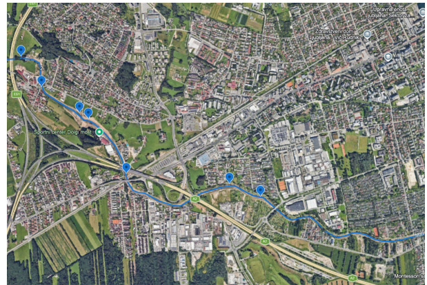
Figure 13. Planned locations for the deployment of button-type temperature sensors at the Gradaščica River.
